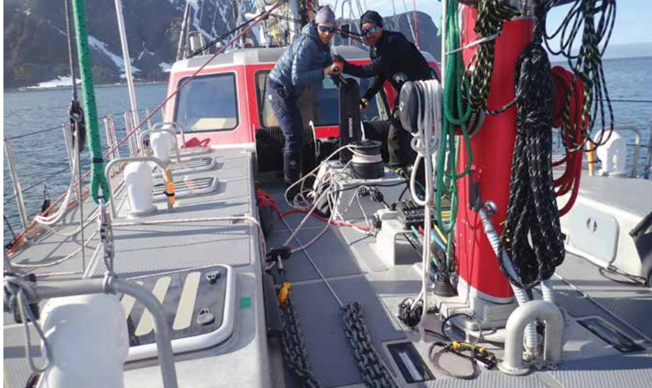
Demonstration of recovering the anchor chain in case of windless failure.
