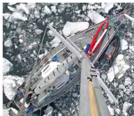
Pelagic is a 54ft (16.5m) steel sloop with a lifting keel and rudder for high-latitude sailing
